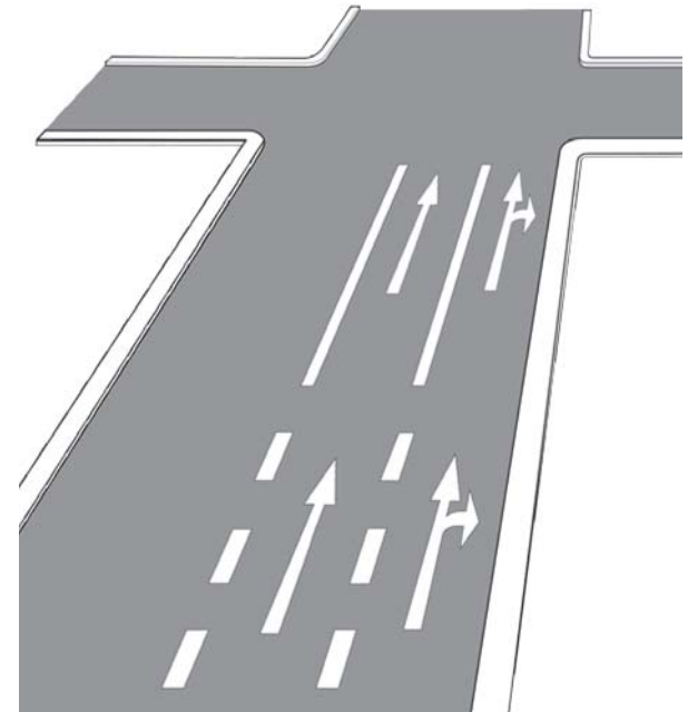
Schematic illustration of a consolidated right turn lane
